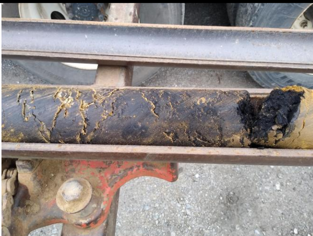
A typical view of a coal seam encountered at 6'-7' below ground surface.
