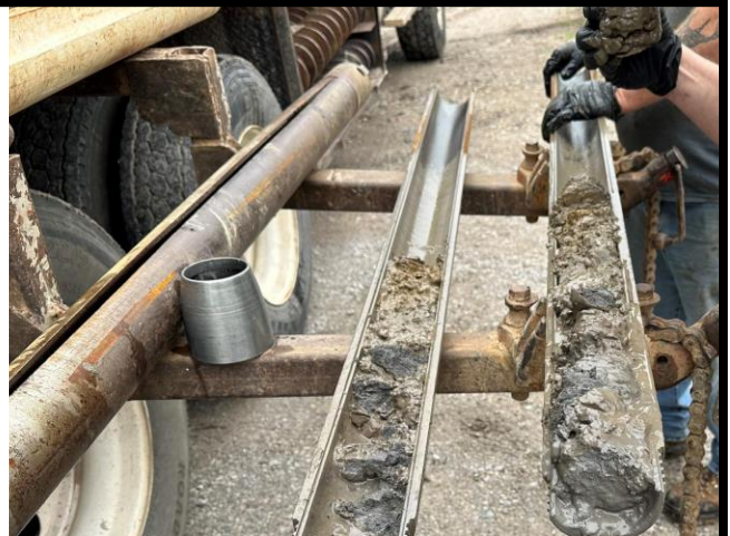
Saturated limestone and shales encountered at 12'-13' below ground surface.
