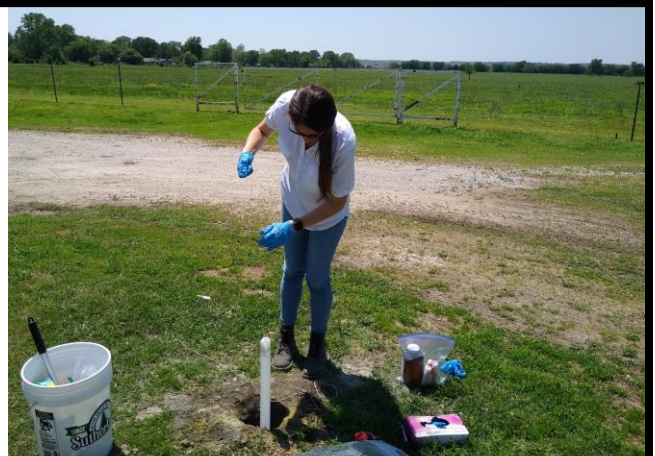
Groundwater sampling with a disposable bailer.
